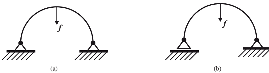
Figure 2: (a) A pre-stressed bearing fosters tangential force flow i.e. bending-stiff membrane behavior. (b) Introduction of a floating bearing significantly reduces the resistance to bending.
