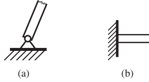
Figure 4: Available boundary conditions: (a) Setting \mathbf{v} = \mathbf{0} on the boundary amounts to a fixed but limp bearing. (b) Enforcing D\mathbf{v}\hat{\boldsymbol{\delta}} = \mathbf{0} , where \hat{\boldsymbol{\delta}} is the outer normal of \Gamma , suppresses rotations around the boundary curve but does not necessarily limit translational degrees of freedom.
